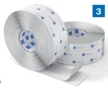
One side is fully adhesive, the other has a fleece layer with a 20 mm wide adhesive strip attached to it. This window connection tape is ideal for creating tight connections of windows or doors **before** installation.
